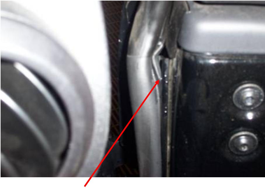
Seal is not seated in channel
