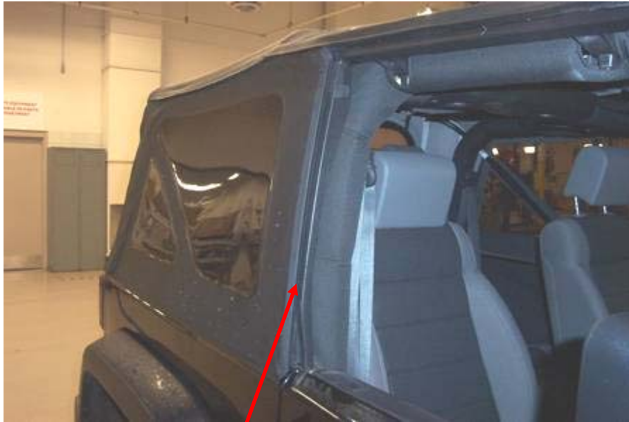
Incorrect – Retainer Not Rolled into Door Rail
