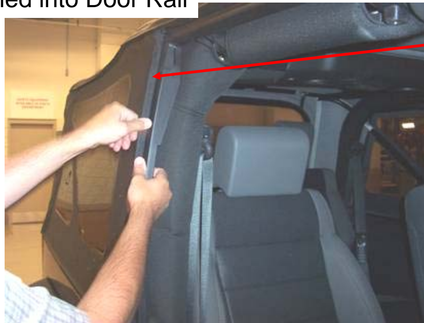
Incorrect – Retainer Not Rolled into Door Rail
