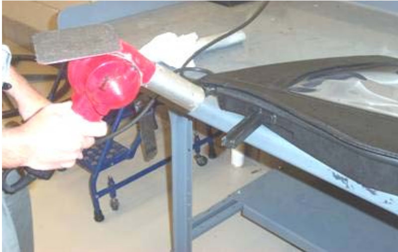
Heat Post: Caution too much heat will melt Door, Maintain 12 inches for 2 Min. Max
